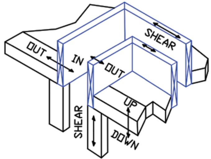
Figure 9 – Expansion joint closure system movements.
