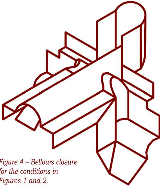
Figure 4 – Bellows closure for the conditions in Figures 1 and 2.
